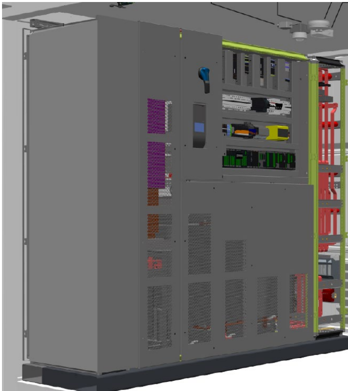
Figuur 5 Omvormer skid Battery mobile 2B
